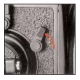
A. For photography with the mirror locked up, first cock the shutter with the film winding crank and, then, turn the mirror lock-up lever in the arrow-indicated direction. The lens shutter will be closed down and the reflex mirror and film safety plate will swing up.
