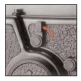
C. Upon completing the multiple-exposed picture, be sure to return the multiple exposure lever counter-clockwise back to its vertical position. Otherwise, there will be an additional multiple exposure on the same frame.
