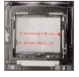
B. When set for multiple exposure, a red warning indicator will appear on the right-central area of the focusing screen.
