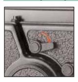
A. To make multiple exposures, first, rotate the film winding crank to advance film, cock shutter and charge mirror action. Then, turn the multiple exposure lever in a clockwise or arrow-indicated direction. The shutter can be released and cocked any number of times, in this condition, without advancing the film.
