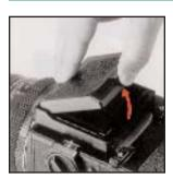
A. The focusing hood of the waist-level finder is opened by pushing or pulling up on the focusing hood/magnifier catch at the rear of the folded waist-level finder.
