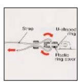
C. Next, thread the neck strap through the plastic ring cover and the U-shaped ring and pull it out, as illustrated.
