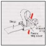
B. Next, insert the U-shaped ring into the slot of plastic ring cover.
