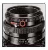
B. Next, cock the shutter with the film winding crank and then shift the time exposure lever to the left (looking from the body towards the lens) which will expose a red-colored "T" on the barrel. The shutter will stay open when the shutter release button is depressed in this condition. The shutter is closed by shifting the time exposure lever in the opposite direction and exposing the letter "A" once more.
