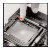
A. The focusing screen can be exchanged, depending on the type of photographic work being undertaken. First, remove the finder attached to the camera main body. Then, move the screen removal lever in the arrow-indicated direction, as illustrated. Finally, lift it up by the lever.
